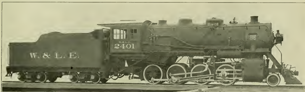
Powerful Consolidation Type Locomotive for the Wheeling & Lake Erie.
